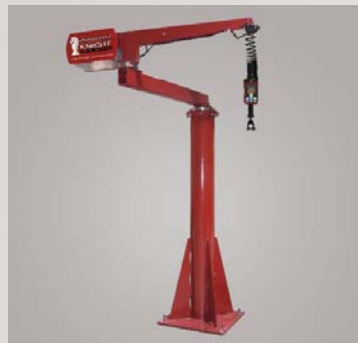
▲ KSHAEA250 Servo Hoist Articulating Extension Arm "Floor Mounted" Articulating Extension Arm attached to a Servo Hoist. Allows for overhead extended non-linear reach within a work cell. May be mounted to a single bridge, rotating carriage, or floor mounted pedestal (250lb/113kg).
