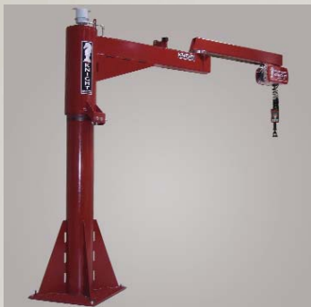
▲ KSHAEA750 Servo Hoist Articulating Extension Arm "Floor Mounted" Articulating Extension Arm attached to a Servo Hoist. Allows for overhead extended non-linear reach within a work cell. May be mounted to a rotating carriage or floor mounted pedestal (750lb/340kg).
